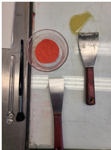
Soft bristled brush, Mason Stain®/Frit 3134 mixture, and tint base ink recipe
